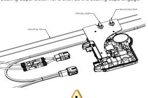
WARNING: Install sealing caps on all unused AC connectors as these connectors become live when the system is energized. ealing caps are required for protection against moisture ingress
