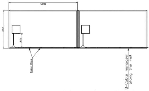
Figure 3: Maxeon 5 AC system landscape layout showing module backside and Q Cable management along module frame using cable clips
