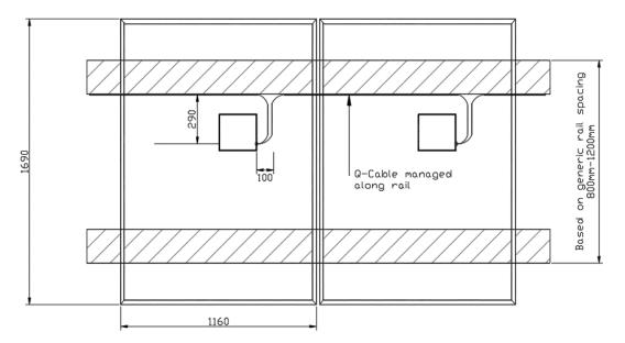
Figure 5: Performance 3 AC Portrait layout showing module backside and Q Cable management For this example, the generic rail placement is 800mm to 1200mm.
