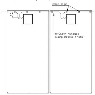
Figure 1: Maxeon 5 AC system portrait layout showing module backside and Q Cable management along module frame using cable clips
