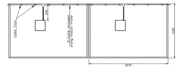
Figure 6: Performance 3 AC system landscape layout showing module backside and Q Cable management along module frame using cable clips
