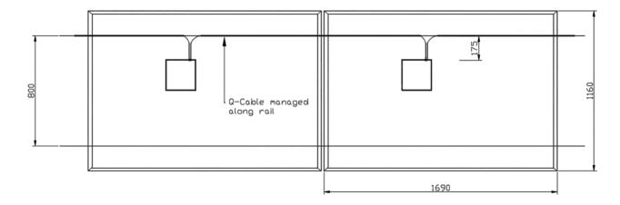
Figure 7: Performance 3 AC system layout showing module backside and Q Cable management along the rail. For this example, the rails are spaced at 800mm apart.
