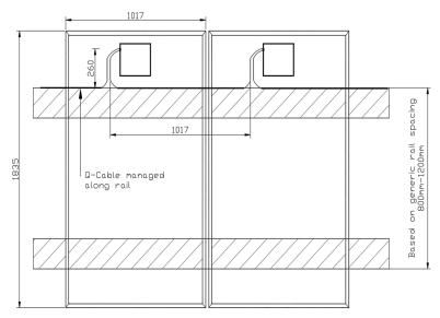
Figure 2: Maxeon 5 AC system portrait layout showing module backside and Q Cable management along the rail
