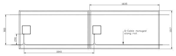
Figure 4: Maxeon 5 AC system landscape layout showing module backside and Q Cable management along the rail
