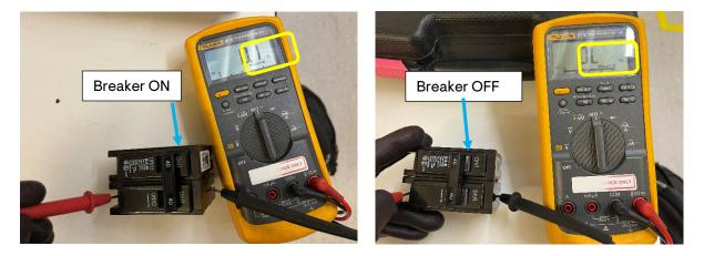
With the breaker in the OFF position, use a multi-meter to check continuity between the screw terminal of the breaker and the breaker contacts that plug into the load center. The multi-meter should indicate OPEN/OL for both the poles if the breaker is in proper working condition.
