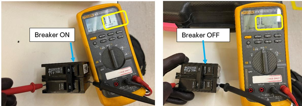
With the breaker in the OFF position, use a multi-meter to check continuity between the screw terminal of the breaker and the breaker contacts that plug into the load center. The multi-meter should indicate OPEN/OL for both the poles if the breaker is in proper working condition.
