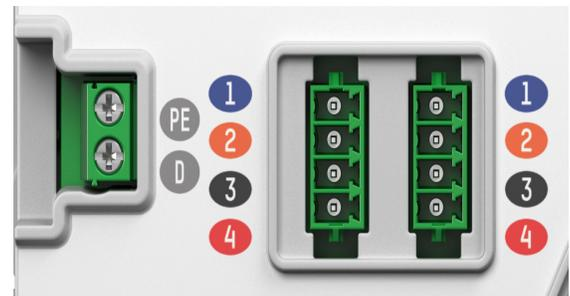
Figure 5: Control header view on control adapter
