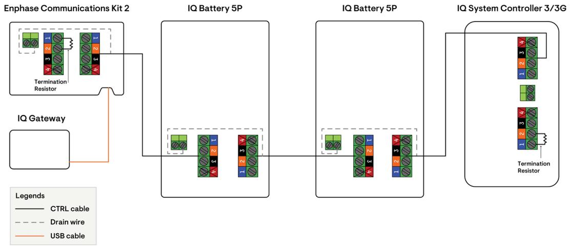
Sequence 3: IQ System Controller 3/3G - Enphase Communications Kit 2 - IQ Battery(s) 5P
