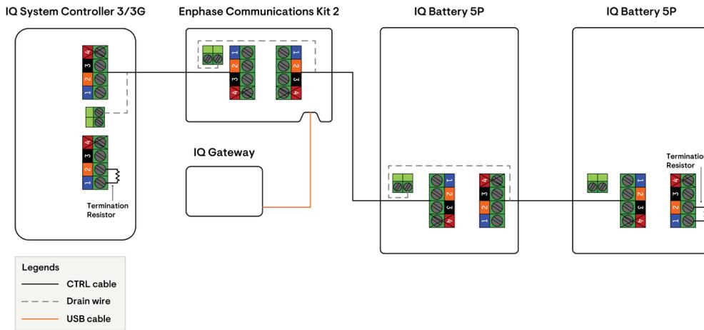
Sequence 4: Enphase Communications Kit 2 - IQ System Controller 3 - IQ Battery(s) 5P
