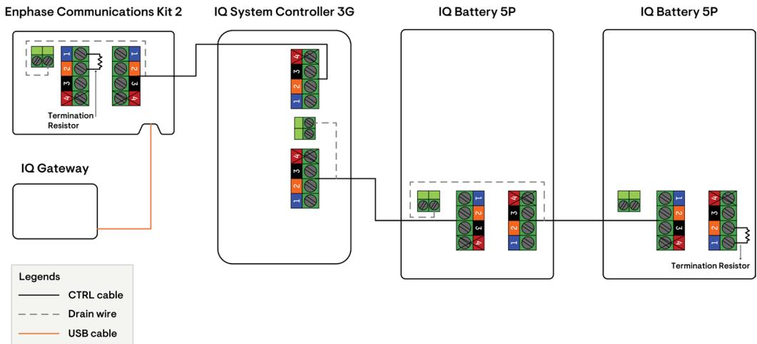
Sequence 2: Enphase Communications Kit 2 - IQ Battery(s) 5P - IQ System Controller 3/3G
