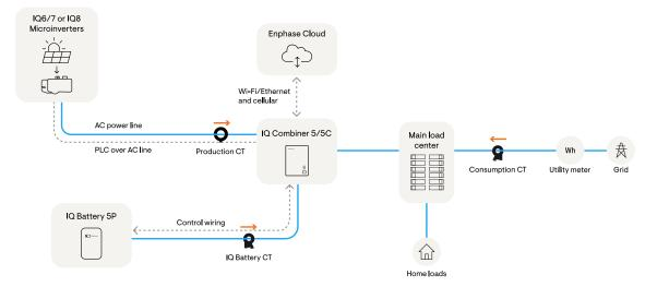
Figure 3: Current transformer installation for grid-tied PV+IQ Battery sites
