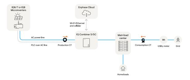
Figure 1: Consumption meters used for net grid metering
