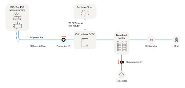
Figure 2: Consumption meters used for home consumption metering
