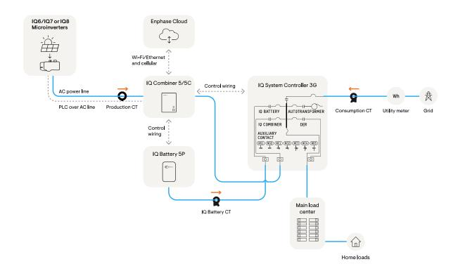
Figure 6: Current transformer installation for Enphase Energy System sites. Whole home backup
