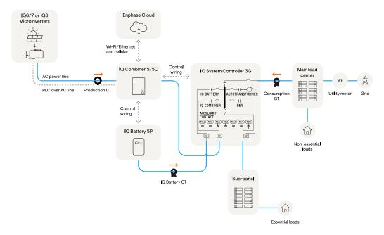
Figure 5: Current transformer installation for Enphase Energy System sites. Partial home backup (With MPU Avoidance)
