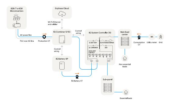
Figure 4: Current transformer installation for Enphase Energy System sites. Partial home backup (No MPU Avoidance)
