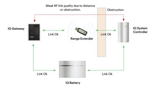
A common use case for installing the ZWRE is shown below. In this site, the IQ Gateway and the IQ System Controller are collocated near the service entrance and the IQ Batteries are installed at a different location often due to harsh weather conditions.
