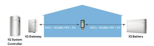
The ZWRE can also be very effective if the direct path between equipment has obstructions such as walls, but the ZWRE provides an alternative path without these obstructions. One example could be sites where the equipment is located on perpendicular walls and do not have line of sight. In these cases, if an appropriate location of ZWRE can be found, then the ZWRE can have a direct line of sight with all the equipment, thereby providing a "hop" with a significantly better RF link quality.
