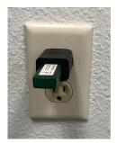
In sites where the IQ Gateway is located far from the IQ Batteries and IQ System Controller, the WUE can be an effective way to improve RF link quality. In WUE, a USB to ethernet receiver and transmitter pair is used to re-locate Communications-kit close to the location of IQ System Controller and IQ Batteries.
