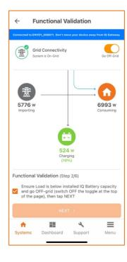
Confirm that the microgrid is operational and loads did not drop. Do this by observing the loads and testing for voltage at the backup panel.
