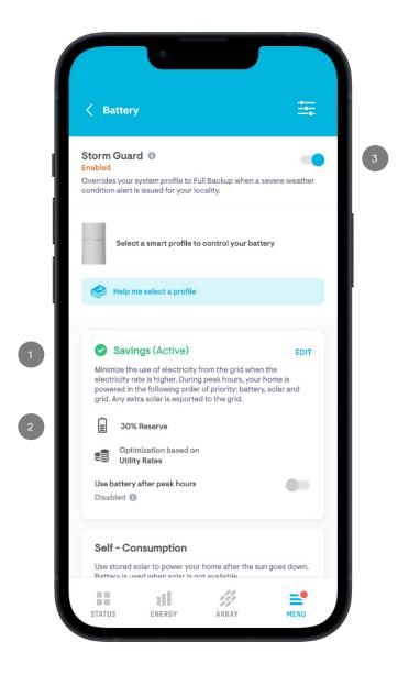
To complete the Savings profile configuration, you will need access to the details of the electric rate schedule for your utility account. You must also decide how much of your IQ Battery 5P capacity will be held in reserve for backup power in case of a grid outage. This is referred to as your reserve capacity.
