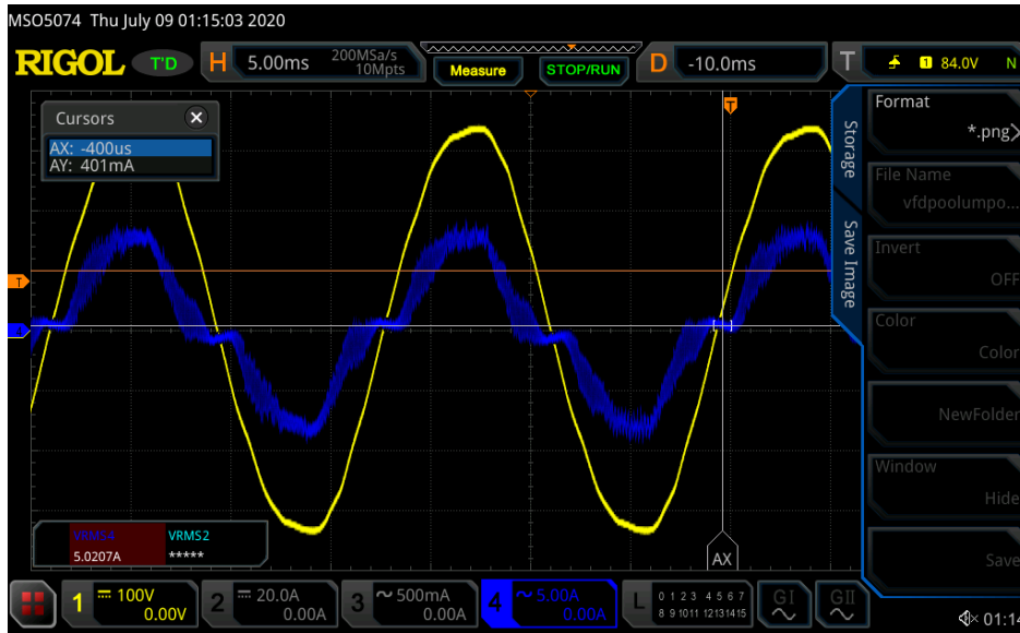
Figure 3: Voltage and current waveforms of an electric motor with VFD. Note the distortions on the current (blue) waveform.
