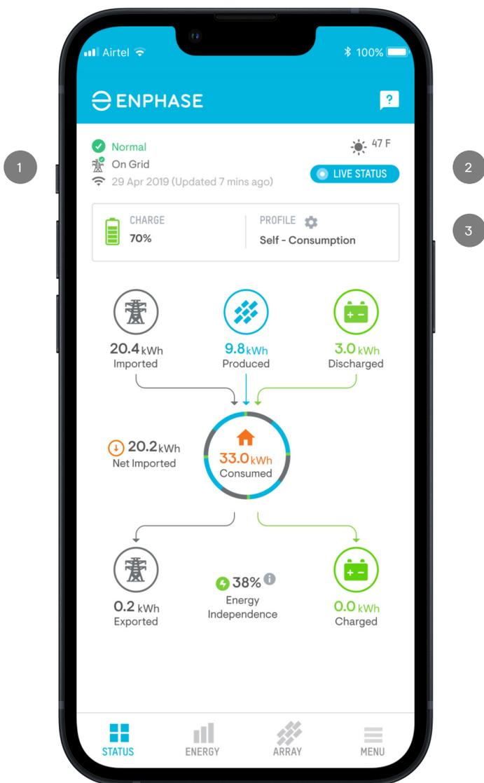
1 In the upper left corner of the Status section, you can see the **operating status** of your system and whether your system is On Grid or Off Grid.
