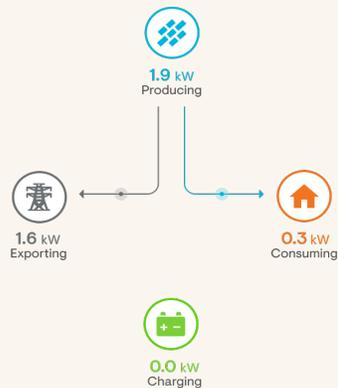
**Solar production powers the home and exports excess power to the grid when the batteries are fully charged.**
