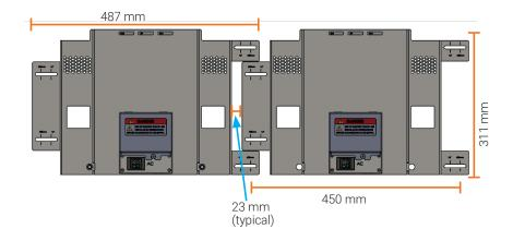
BWM-600MM-A allows 600 mm battery-to-battery spacing:
