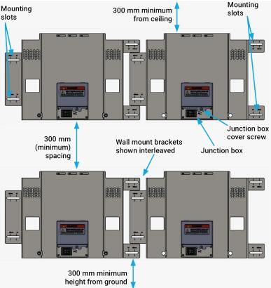
If installing additional batteries, install the adjacent wall-mount brackets in an interleaved fashion, as needed. Be sure to align the mark on the adjacent wall-mount bracket to the centre of the wall stud. A small gap in between the adjacent wall-mount brackets is normal. You may install another row of wall-mount brackets above the one already installed. Maintain at least 300 mm (one foot) clearance between rows.
