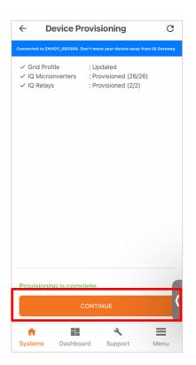
**NOTE:** After provisioning is complete, the IQ Microinverter takes around 20-30 minutes to start production.
