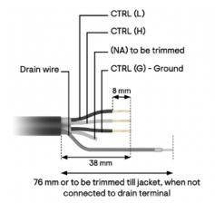
Wire the Control/CTRL cable in a daisy chain, connecting the IQ System Controller, first IQ Battery 5P, and second IQ Battery 5P. The following image shows the IQ System Controller's Control/CTRL cable termination.
