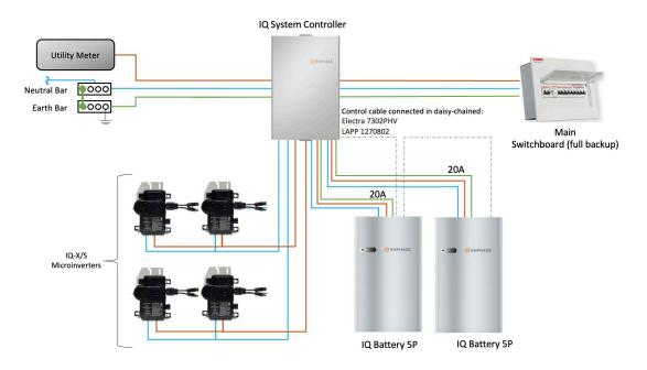
Recommended MCB for each microinverters branch is 25 A, and the minimum PV submains are 6 mm<sup>2</sup> each.
