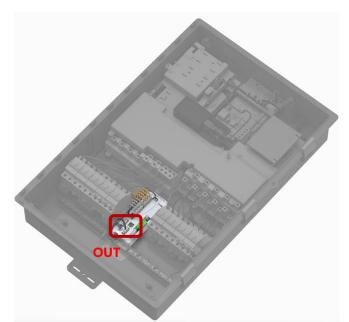
The following image shows the IQ Battery 5P Control/CTRL cable terminations. Note that the IN and OUT labels on the IQ Battery 5P Control/CTRL board must be wired in the correct order.
