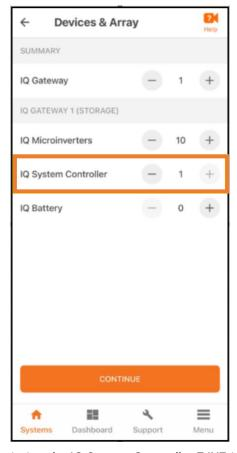
To successfully install and commission the IQ System Controller 3 INT, it is mandatory to have the Enphase Installer App version V3.34.3 or higher. Ensure this requirement is fulfilled by checking the **Menu** tab and updating via the Apple App Store or Google Play Store.
