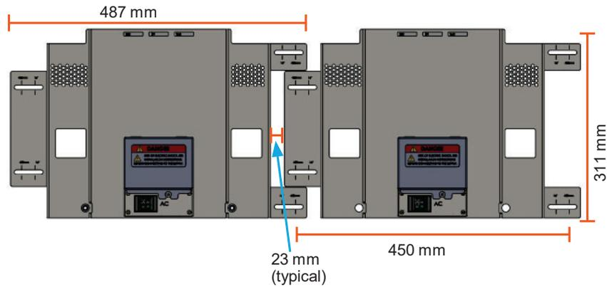
BWM-600MM-A allows 600 mm battery-to-battery spacing:
