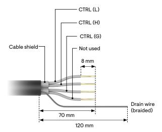
The tested and supported **control cable** make is **Belcom** and model is **4302P2254-01**.
