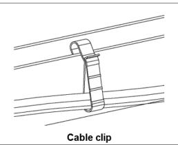
Dress any excess cabling in loops so that it does not contact the roof. Do not form loops smaller than 12 cm  $(4\frac{3}{4})$  in diameter.
