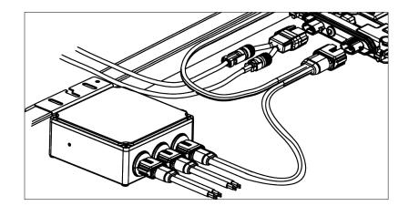
A. Cover any unused connectors with IQ Sealing Caps. Listen for a click as the connectors engage.
