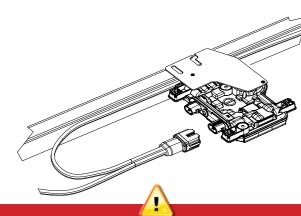
WARNING: Install sealing caps on all unused AC connectors as these connectors become live when the system is energised Sealing caps are required for protection against moisture ingress.
