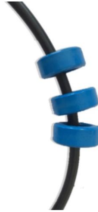
Figure 7: Multiple Toroid Rings Fitted on a Larger Core Cable
