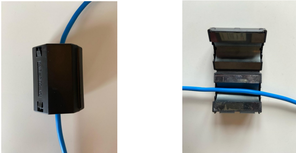
Figure 9: Gapped ferrite core on the neutral conductor with the 3M Kapton tape applied between the two parts of the ferrite core
