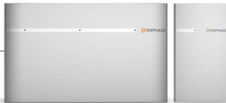
IQ Battery 3T / 10T 10 kVA grens: maximaal (7x3T) of (2x10T+1x3T) Monofasig: maximaal 3x3T OF 1x10T
