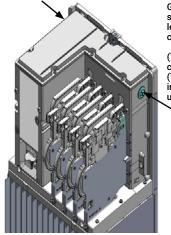
Grommet to be installed on the left side or right side when the hole in the left side or right side is not used for cable routing.
