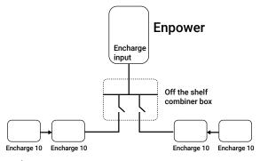
⚠ WARNING! Parallel power production sources only. Do not connect load circuits.
