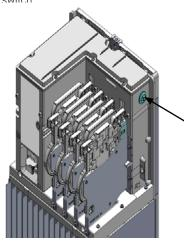
Grommet to be installed when the hole in the indicated location is not used for cable routing.
