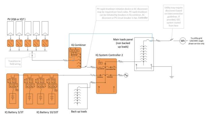
Figure 6: Enphase Energy System in Home Essentials configuration with M-Series Microinverters & System Controller 1.
