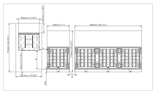
Figure 20: Bracket spacing for IQ Battery 3T or IQ Battery 10T
