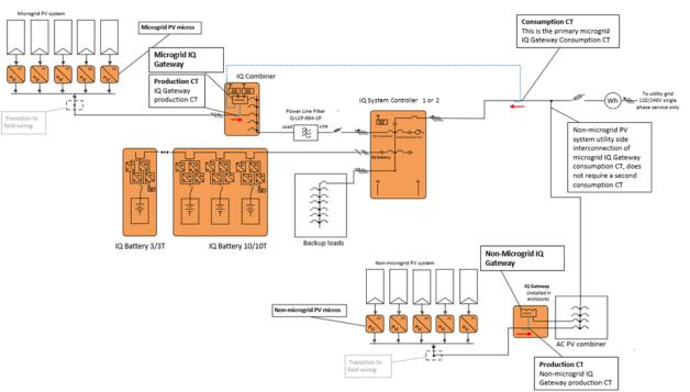
Figure 15: "Split" PV system that does NOT require an additional set of Consumption CTs
