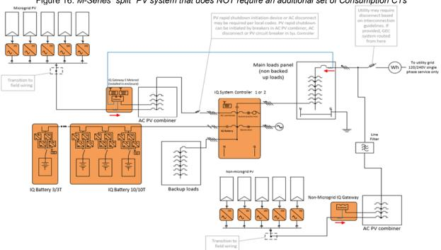
Figure 16: M-Series "split" PV system that does NOT require an additional set of Consumption CTs
