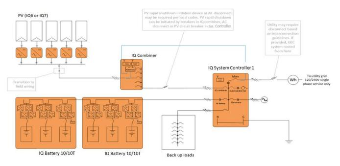
Figure 10: Enphase Energy System in Full Energy Independence configuration with IQ6 or IQ7 Microinverters & System Controller 2.
