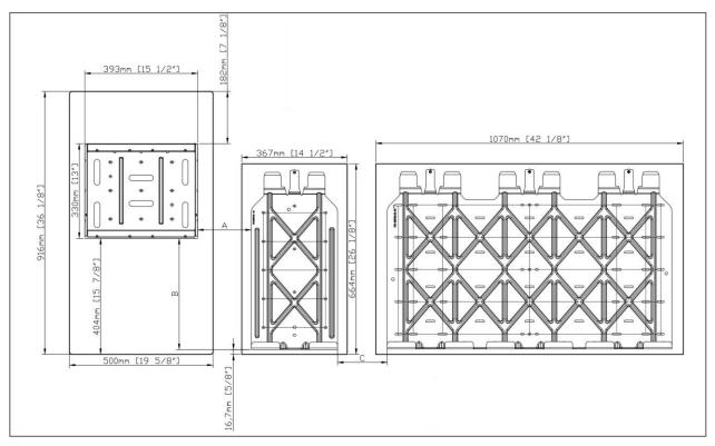
Figure 19: Bracket spacing for IQ Battery 3 or IQ Battery 10
