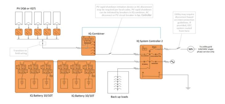
Figure 11: Enphase Energy System in Full Energy Independence configuration with M-Series Microinverters & System Controller 1.
