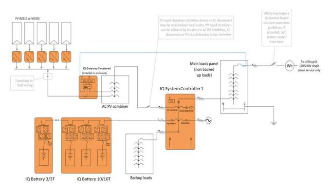
Figure 7: Enphase Energy System in Home Essentials configuration with M-Series Microinverters & System Controller 2.
