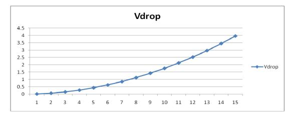
Since the voltage drop is non-linear, reducing the number of Microinverters in the branch circuit greatly reduces the voltage measured at the last Microinverter in the branch. One way to minimize this voltage drop is to "center feed" the branch. The diagram below illustrates the "center fed" method.
