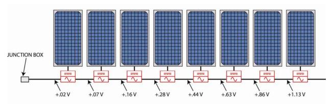
As Microinverters are added to the branch circuit, the voltage drop increase is non-linear. The graph below illustrates how the voltages measured at the individual Microinverters increase in a fully populated branch circuit of 15 M190 Microinverters.
