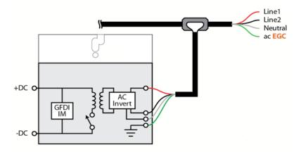
**Enphase Microinverters with Integrated Ground: Ground Connections**
