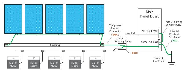
Enphase Microinverters with Integrated Ground with EGC Connecting PV Frames and Racking
