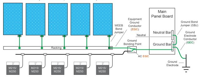
Enphase Microinverters with Integrated Ground with WEEB Ground Jumpers
