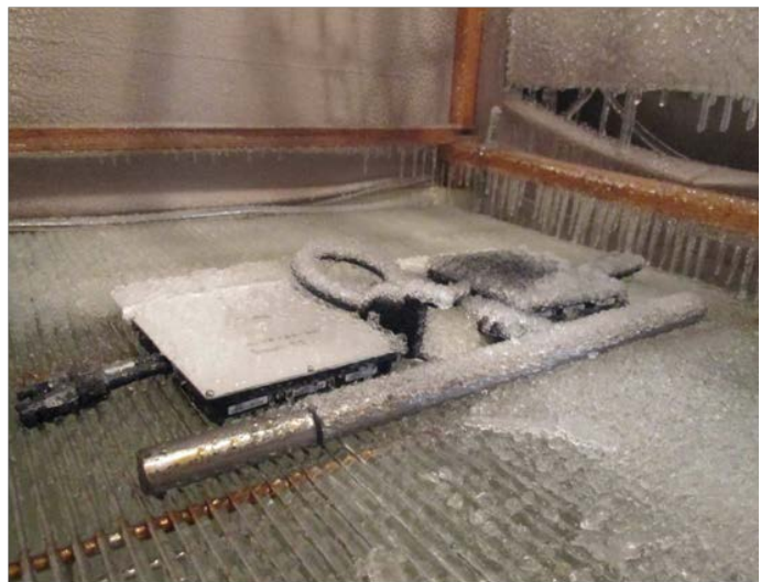
View of the Enphase M250 Microinverter undergoing the test for ingress of water (left) and the external icing test (right). Both tests were performed by an accredited, independent laboratory.
